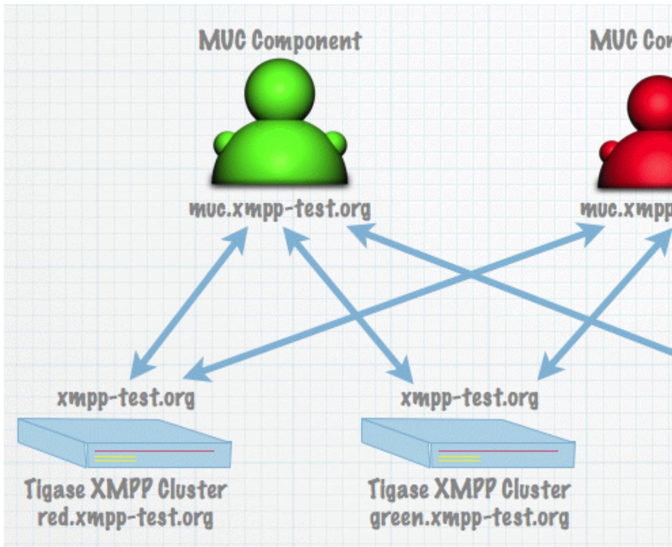
We want to make it possible to connect the MUC component to all nodes. To do so, we are configuring Tigase XMPP Server to run in the cluster mode and on each of cluster nodes we need to enable `ComponentProtocol` component.
