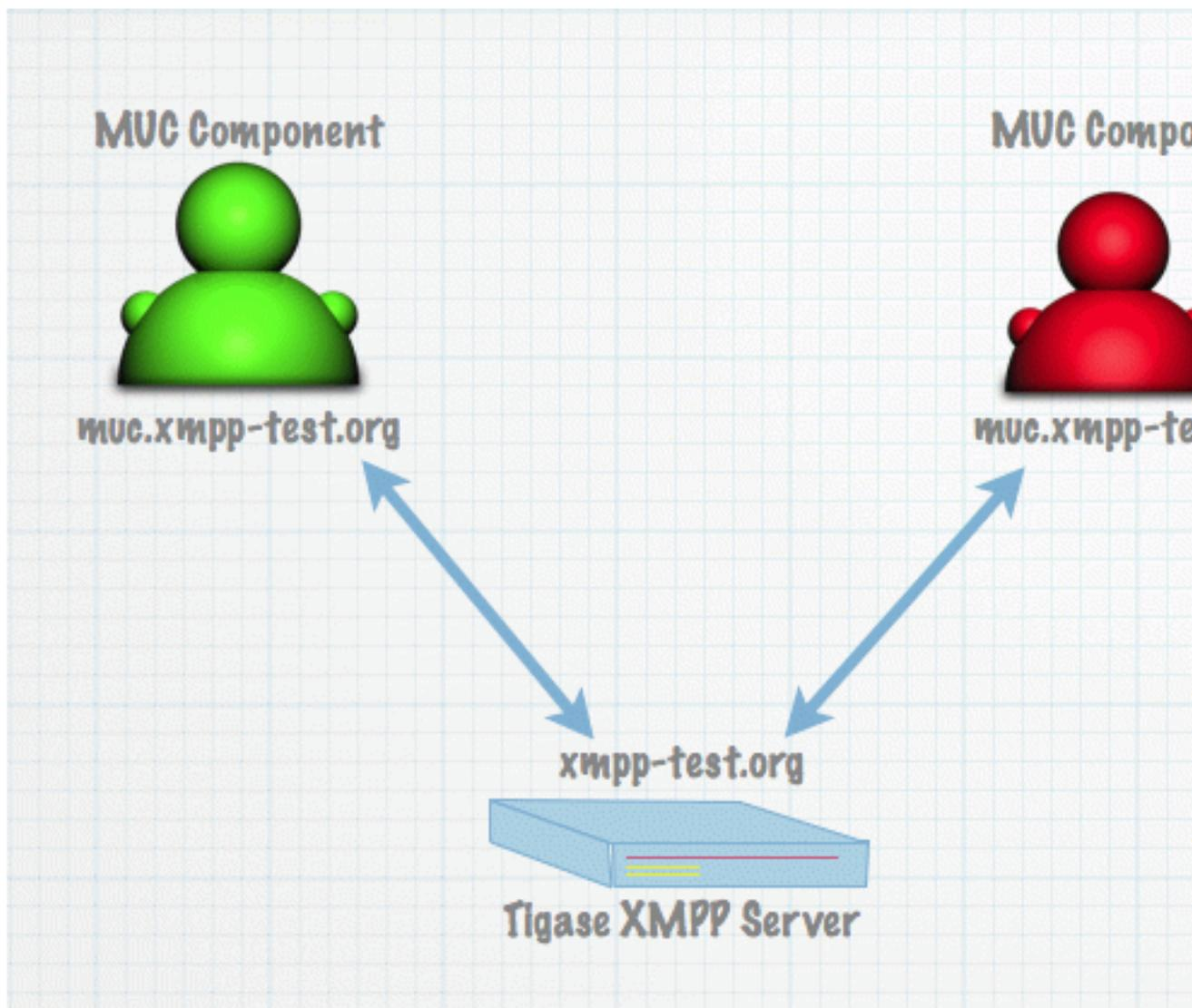
We have a single machine running Tigase XMPP Server and 2 instances of the MUC component connecting to Tigase.
